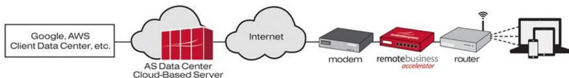
Each RBA works in conjunction with the cloud, reducing and optimizing traffic. Data flowing through the RBA is inspected in blocks; each block consists of 4,000 bytes. As each 4K block passes through the cloud or the RBA, its pattern is recognized and committed to memory. A unique data character is sent in lieu of sending data blocks that have been previously sent, thereby reducing data traffic.
