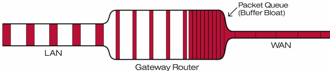
When bursts of data arrive at a router, the excess data queues up in the buffer. If the queue becomes too great, time sensitive packets, such as Voice over IP (VoIP) and video, get buried in the buffer, thereby causing garbled voice conversations and tiling in a video presentation.
